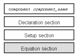
The equation section of a Simscape file follows the declaration and setup sections. It is executed throughout the simulation. The purpose of the equation section is to establish the mathematical relationships among a component's variables, parameters, inputs, outputs, time and the time derivatives of each of these entities.
